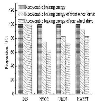
Fig. 3.3 Impact of hydraulic pump/motor configuration on braking energy regeneration.
